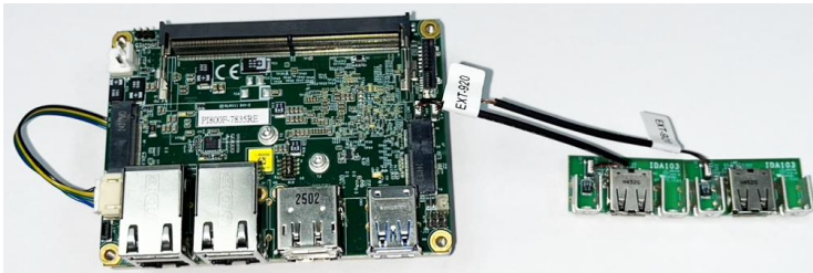
The picture shows EXT-920 cables connected to the J15/J16 headers and to the IDA103 USB 2.0 modules
