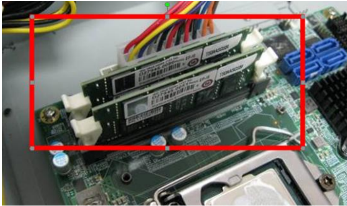
Figure 2-6. DDR4 SO-DIMM Memory Installation Steps:
