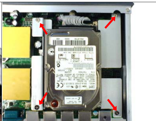
Fig. 8-4 Fix all four screws back
