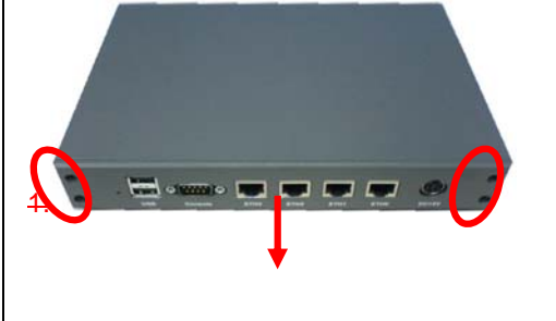
Fig. 5-1 Loosen the four screws of the chassis on the back to remove the top lead.
