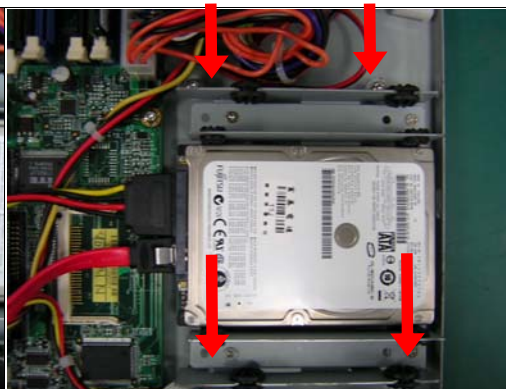
Fig. 10-6 Fixed HDD bracket and Fix two screws back
