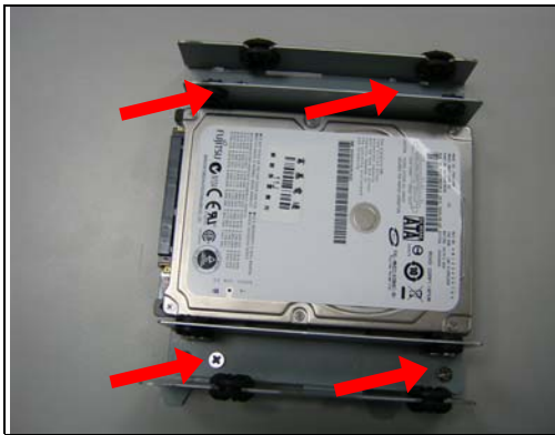
Fig. 10-3 Fasten the four screws to lock 2.5" HDD and bracket together.
