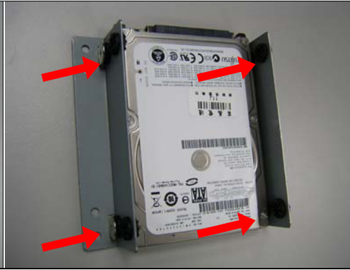
Fig. 10-2 Fasten the four screws to lock 2.5" HDD bracket and bracket together.
