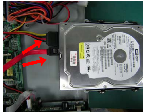
Fig. 9-3 Connect SATA cable and power connector to 3.5" HDD
