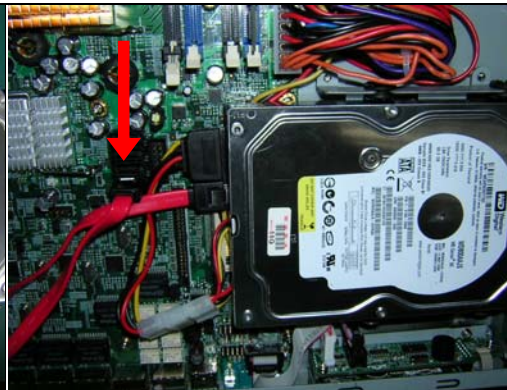
Fig. 9-4 Connect SATA cable to MB935
